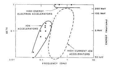
Figure 1: Phase velocity vs frequency of the superconducting cavities which are in use or at the advanced development stage
