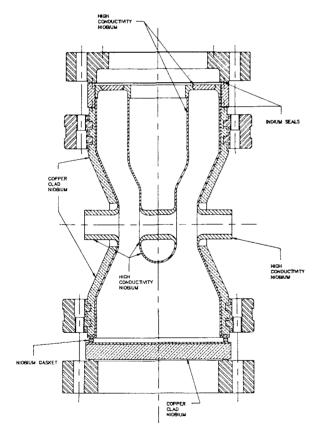
Figure 3: Coaxial quarter-wave resonator; 425 MHz, 0.155 c  $\,$
