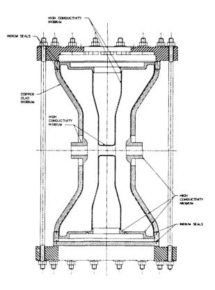
:.gure 4: Coaxiai half-wave resonator; 425 mmz, 0.18 c
