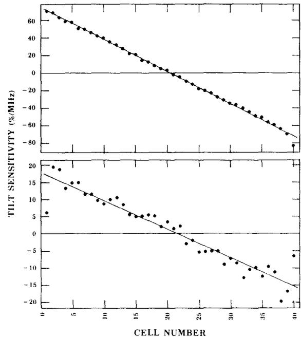
Fig. 1. Tilt sensitivity without post couplers for the 1.84-m-long, 40-cell DTL. The upper plot corresponds to single stems and has a slope of  $-80\%/MHz/m$ . The lower plot corresponds to double stems  $180^\circ$  apart, with a slope of  $-18\%/MHz/m$ .
