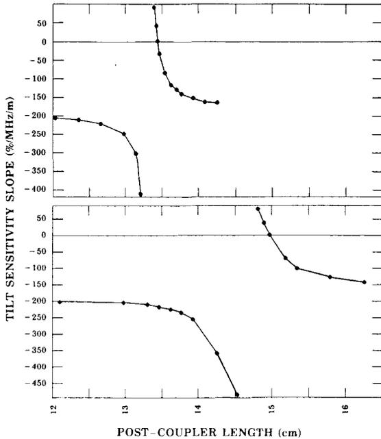
Fig. 2. Tilt sensitivity slope versus post-coupler length for the 3.54-m-long, 16-cell DTL equipped with single stems. The upper plot corresponds to seven post couplers, one every other drift tube. Stabilization (zero TS slope) occurred for a post-coupler length of 13.4 cm. The lower plot corresponds to 15 post couplers, one every drift tube. Stabilization occurred at 15.0 cm.
