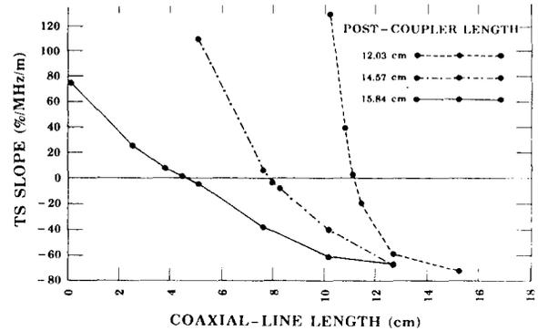
Fig. 6. Tilt-sensitivity slope versus post-coupler coaxial-line length for the 3.54-m-long, 16-cell DTL with double stems and 15 coaxial post couplers. The three post-coupler lengths refer to inner lengths, that is, inside the tank radius.
