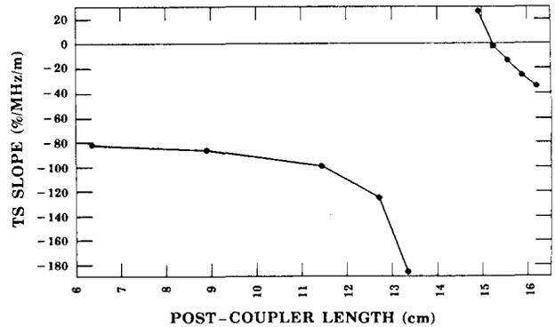
Fig. 3. Tilt-sensitivity slope versus post-coupler length for the 1.84-m-long, 40-cell DTL equipped with single stems and 19 post couplers. Stabilization occurred at 15.3 cm.
