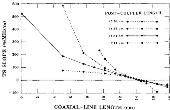
Fig. 5. Tilt-sensitivity slope versus post-coupler coaxial-line length for the 1.84-m-long, 40-cell DTL with double stem and 19 coaxial post couplers. The four post-coupler lengths refer to inner lengths, that is, inside the tank radius.
