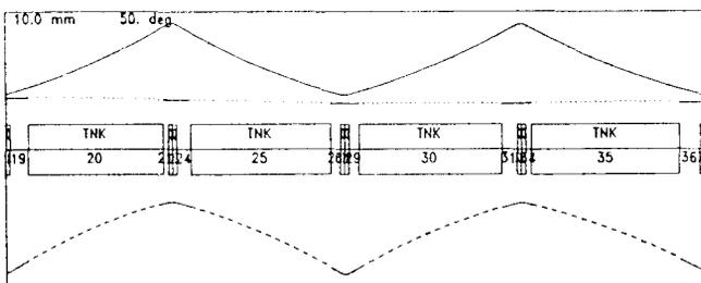
Figure 3: One module of linac structure consisting of two FODO focusing cells
