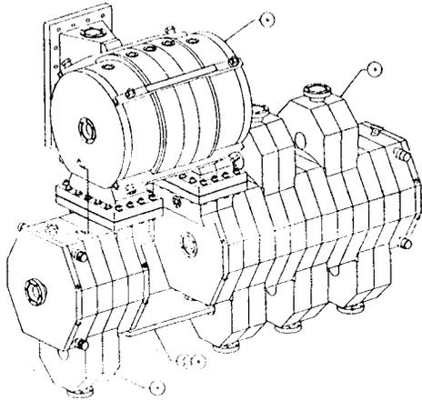
Figure 1: Side-coupled accelerating structure and  $3\lambda/2$  bridge coupler, isometric view (LASL drawing)
