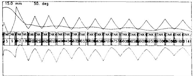
Figure 5: Beam envelopes of linac with power optimized rf gradients using untrimmed values of quads found for  $\Delta E/\Delta L = \text{const.}$
