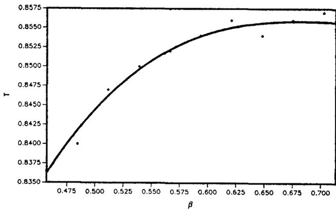
Figure 2: Effective shunt impedance  $ZT^2$  and  $E_m$ , maximum surface field for 1 MV/m axial field, (above) and transit time factor  $T$  (below) as functions of  $\beta$
