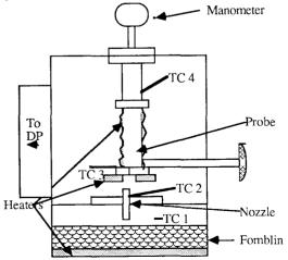
Figure 2. Setup used for Fomblin nozzle tests.
