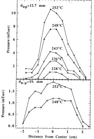
Figure 3. The pressure profile measured for a 4.76 mm (3/10') diameter nozzle at distances of a) 12.7 mm (1/2'') and b) 19.0 mm (3/4'') above the nozzle. For each distance, profiles are measured at several oil temperatures.
