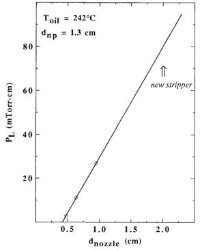
Figure 4. The integral of the pressure profiles as measured in Fig. 3. as a function of nozzle diameter for a fixed oil temperature of 242 °C and distance from the nozzle to the probe of 12.7 mm. The arrow denotes the length of the slit used in the final stripper design.
