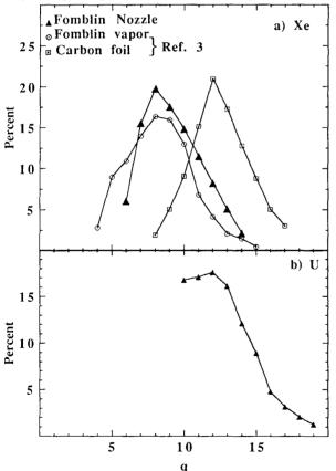
Figure 5. Measured charge state distributions using the final nozzle configuration, a 19.0 mm x 9.5 mm (3/4" x 3/8") slit 5 cm long. a) gives the charge state distribution measured for 131Xe from the present work (4), 136Xe using Fomblin as a stripper (c) and 136Xeusing a solid carbon stripper ( $_{\Box}$ ) (from Ref.3) 5b) gives the measured charge state distribution for <sup>238</sup>U.
