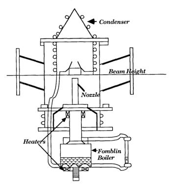
Figure 6. Schematic diagram of new stripper being installed in the MEBT line of the Abel injector at the SuperHILAC.
