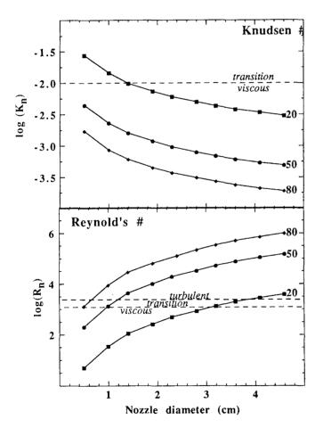
Figure 1. The calculated Knudsen number,  $K_n$ , and Reynold's number,  $R_n$ , as a function of nozzle diameter for three guesses for the diameter of the Fomblin molecule. The three regions of hydrodynamic flow are shown.
