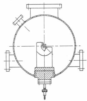
Fig. 6 Cross section of the 4-Rod RFQ
