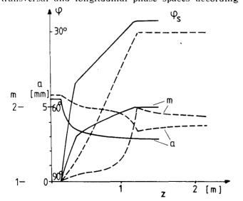
Fig. 3 The variation of the electrode parameters synchronous phase  $\phi_S$ , modulation m, and aperture a along the z-axis. The dashed lines correspond to the standard method of RFQ design and the solid lines Fig. 4 Calculated phase space plots for the beam to the new method used in our design.
