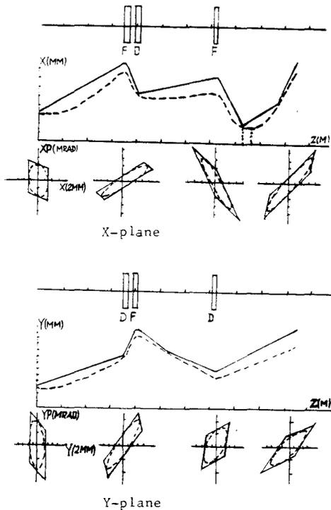
Fig.3. Comparison between the two beam envelopes of example 2.
