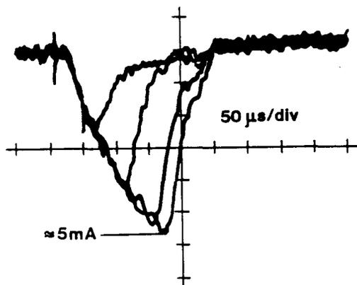
Fig. 4 : Accelerated beam for discharge lengths of 50, 100, 150, 175  $\mu$ s. Source parameters constant.
