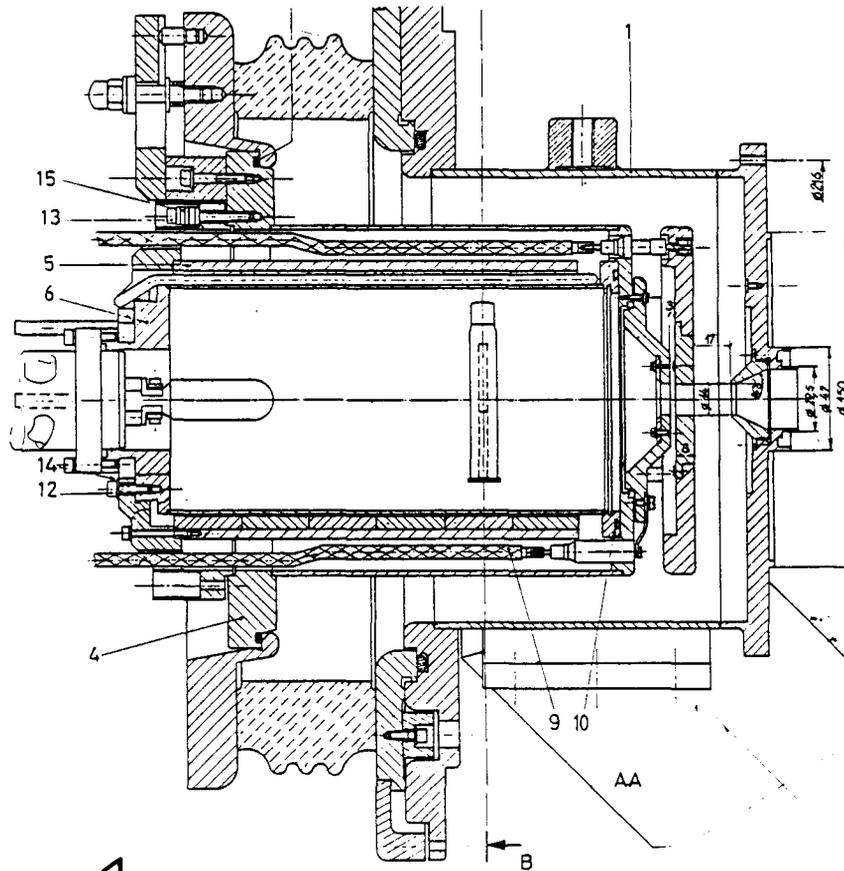
Fig. 1 : Ion source installed in preinjector
