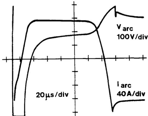
Fig. 2 : Arc voltage and current under optimal conditions.
