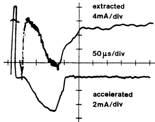
Fig. 3 : Typical beam extracted at 50 kV showing initial electron peak and beam accelerated by the RFQ.
