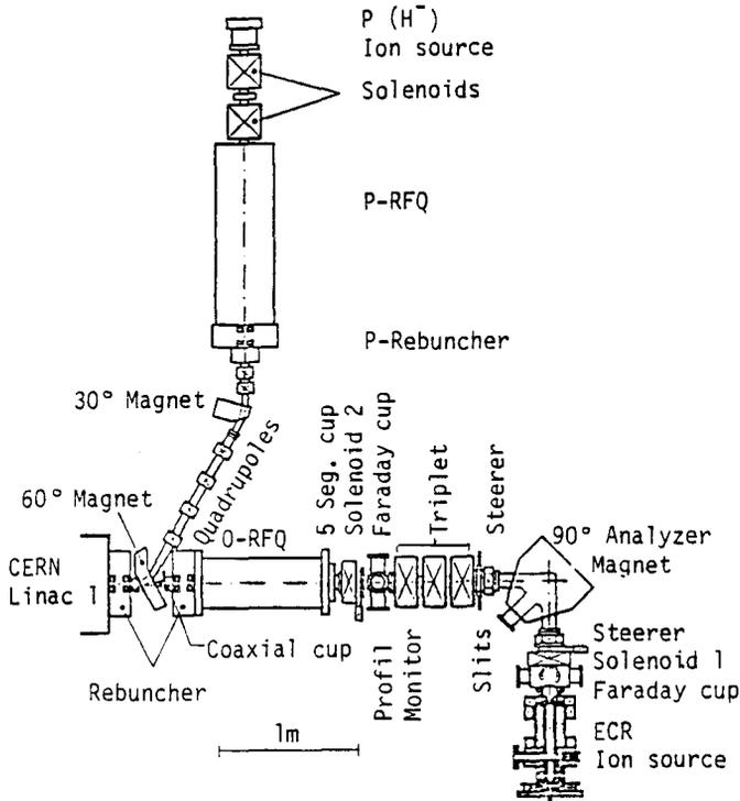
Care has been taken to make the change over from oxygen to proton ( $H^+$ ) injection very rapidly. First ideas involved dis- and remounting of the corresponding RFQ's and major reshuffling of larger components. The present scheme makes it (almost) possible to change over from oxygen to protons and vice versa in between subsequent pulses.
