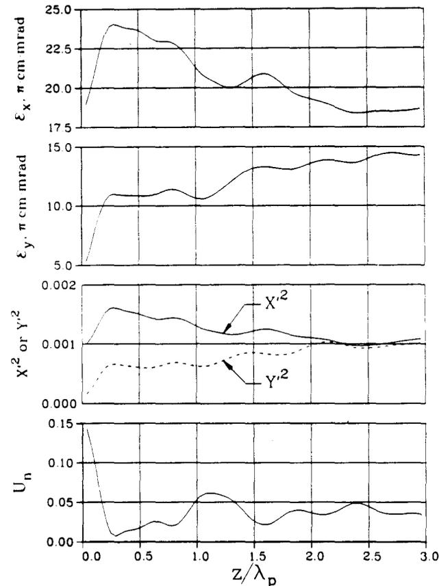
Fig. 1. Variation of beam parameters vs number of plasma periods for initially Gaussian beam,  $P_i = 8$ ,  $k_{xi}/k_{ox} = 0.3$ ,  $(\epsilon_x/\epsilon_y)_i = 4$ ,  $X/Y = 1.41$ .
