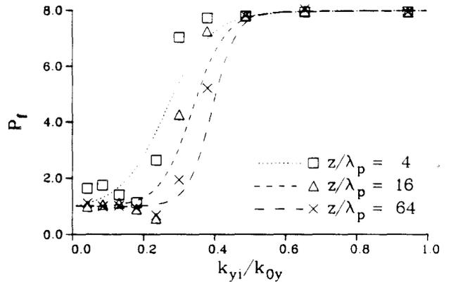
Fig. 5. K-V beams; simulations (data points) and curves from Eq. (3) (dotted lines);  $(\epsilon_x/\epsilon_y)_i = 4$ ,  $X/Y = 1.41$ .
