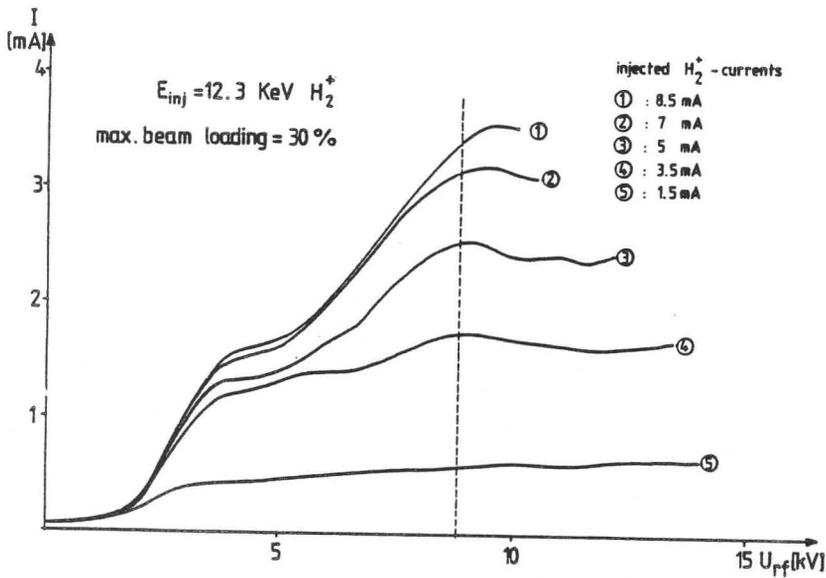
Fig. 8 Transmitted  $H_2^+$  - current versus RF-voltage at different injection currents
