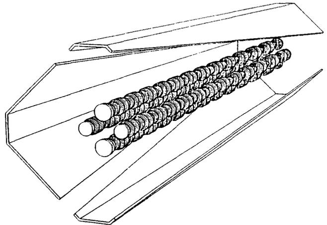
Fig. 1 Trapezoidally modulated SCR-RFQ electrodes
