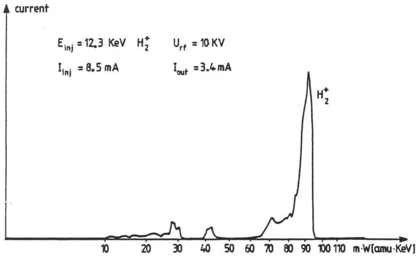
Fig. 7 Measured energy spectrum of an accelerated  $H_2^+$  - beam
