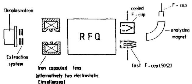
Fig. 3 Scheme of the experimental set up of the SCR - four rod RFQ
