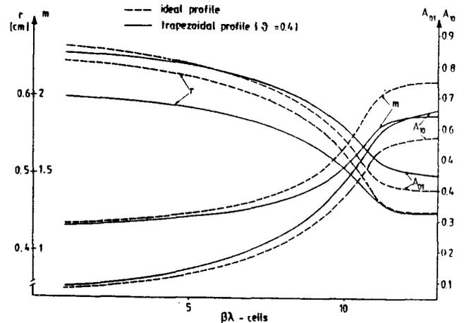
Fig. 2 Coefficients of ideal and trapezoidal ( $\mathcal{D} = 0.4$ ) electrode profile versus section number ( $\beta\lambda$ ) of the SCR-RFQ
