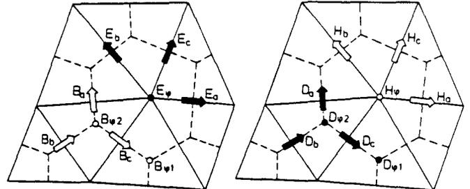
Figure 1 : Allocation of the field components
