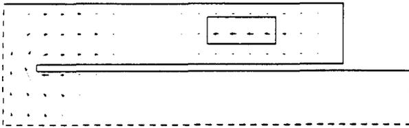
Figure 8 : Magnetic field at  $\varphi = \pi/2$  for the mode 1-EE-2 with  $f=599.10$  MHz.
