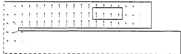
Figure 6 : Electric field at  $\phi = 0$  for the mode 1-EE-1 with  $f=417.17$  MHz.
