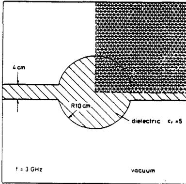
Figure 9 : Dielectric waveguide with mesh for the part which is essential for a run of URMEL-T
