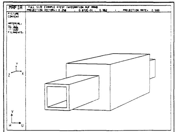
Figure 2: M3 plot of example 1 (retangular pillbox with beamports).
