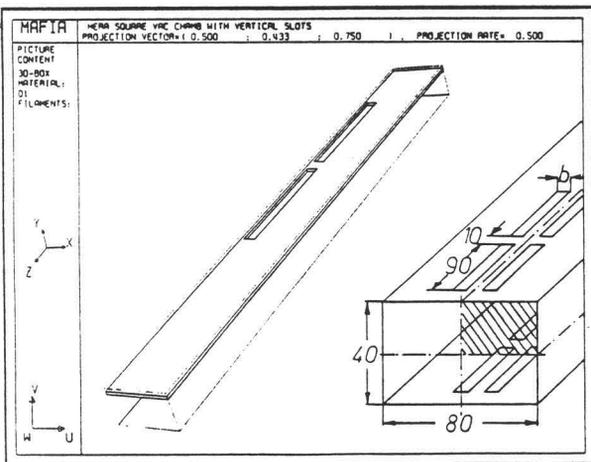
Figure 11: One quarter of HERA square vacuum chamber with vertical slots.
