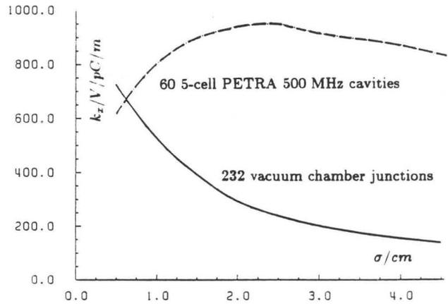
Figure 6: Vertical kick (averaged over the bunch) for 232 vacuum chamber junctions (figure 5) in PETRA in comparison with the kick due to 60 PETRA cavities.
