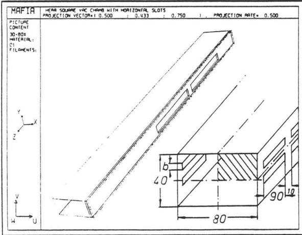
Figure 9: One quarter of HERA square vacuum chamber with horizontal slots.
