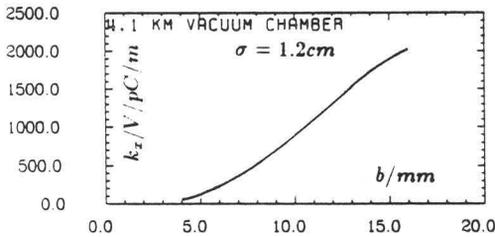
Figure 10: Vertical kick (averaged over bunch) against slot high b for 4.1km structure (figure 9).
