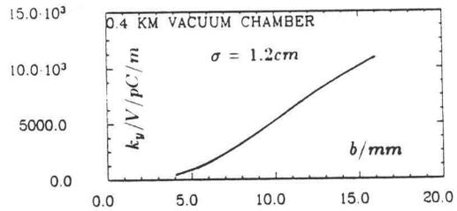
Figure 10: Vertical kick (averaged over bunch) against slot high b for 0.4km structure (figure 11).
