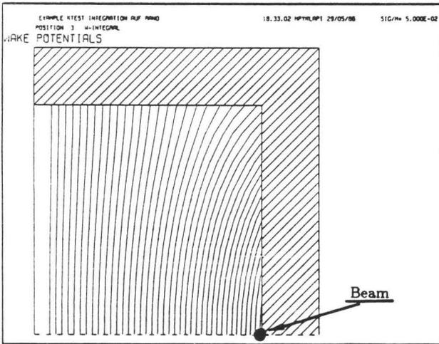
Figure 4: Scaling function  $\int_{-\infty}^{\infty} ds \lambda(s) G(x, y, s)$  for  $k_{||}$  computed by T3 for a rectangular pillbox with beam offset in horizontal direction.
