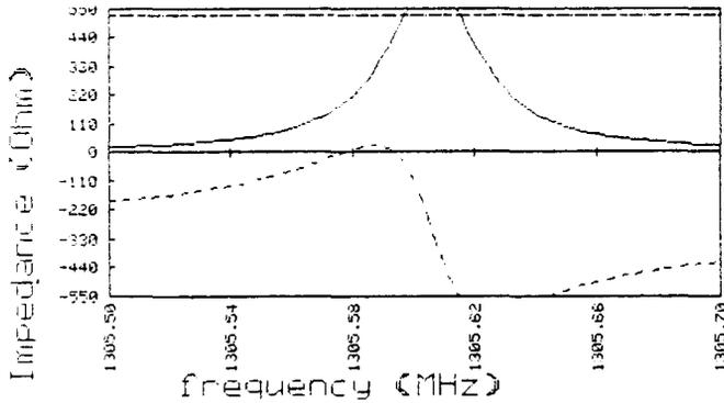
Figure 6: Same plot as previous figure, with open and short circuited frequencies moved 20 kHz further from each other.
