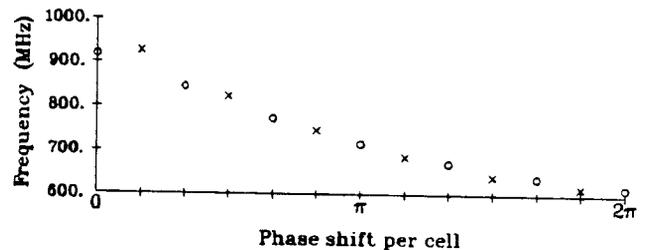
Figure 2: The calculated Jungle Gym dispersion curve
