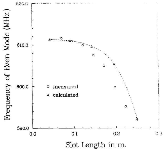
Figure 4: Computed and measured values of the lowest mode of the coupled-cavity system
