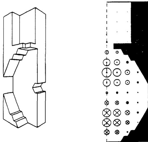
Figure 8: One quarter of the waveguide-cavity system and the electric field plot of the  $TM_{110}$  mode
