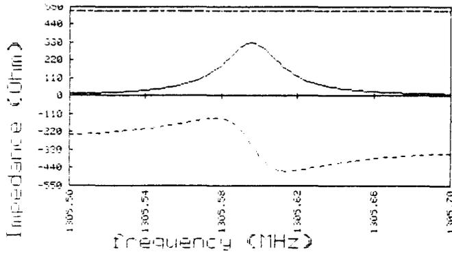
Figure 5: Input impedance to waveguide as a function of frequency near the  $TM_{110}$  resonance of the pillbox cavity. The real part of the impedance is shown solid, the imaginary dashed. The waveguide characteristic impedance is shown with a dot-dash pattern near the top of the figure.
