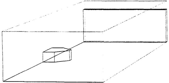
Figure 3: One fourth of one of two cavities coupled by a slot
