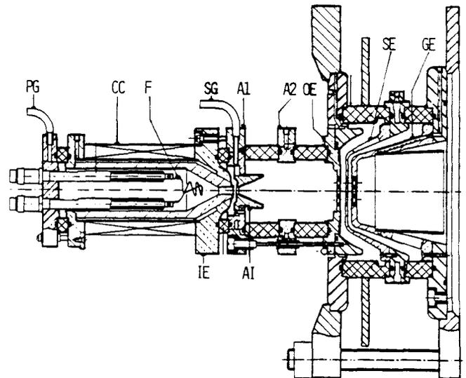
Fig. 1. DUOPIGATRON ion source for oxygen, after Ref. 7. PG, primary gas inlet (argon). CC, compressor coil. F, cathode filament made from rhenium wire. IE, intermediate electrode. SG, secondary gas inlet (oxygen). A1, first anode. AI, anode insert. A2, second anode. OE, outlet electrode. SE, screening electrode. GE, ground electrode. These last three electrodes form a multi-aperture triode (accel/decel) extraction system.
