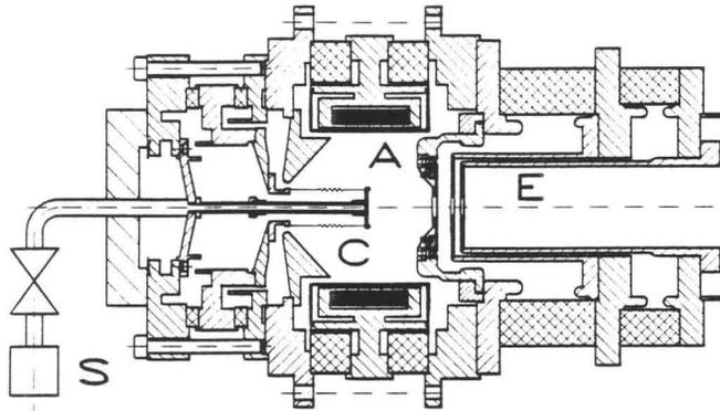
Fig. 2. Hot-running ion source of the CHORDIS type<sup>8</sup> with external supply bottle. A, anode: the inner tube runs hot; the outer, cold wall is lined with 18 permanent magnets producing a linear multi-cusp field for stable plasma confinement. The electrodes that axially enclose the discharge chamber are usually connected to the negative cathode leg. C, cathode made from six tantalum filaments. E, extraction system; single- or multi-aperture triode or pentode. S, vapour supply bottle.
