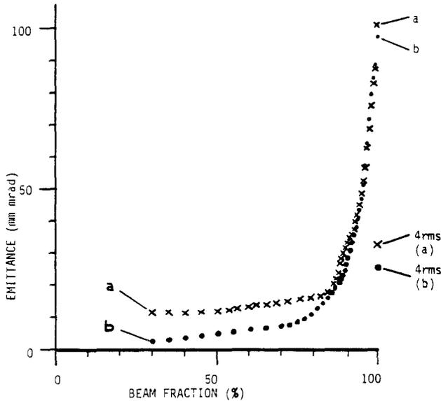
Fig. 10. Beam fraction versus minimum-ellipse size for two different beams simulated by using the code SNOW.<sup>13</sup> The plot shows that case (b) is much more favourable than case (a) because for 75 % and lower beam fractions the emittance values of (b) are only half as large as those of (a), even if both values for the 100 % fractions are nearly identical. On the other hand, the 4rms values of the entire distributions differ by only 20 %. After Ref. 6.
