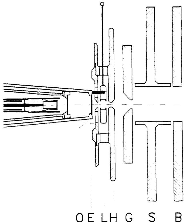
Fig. 7. Compound extraction system for MEVVA.<sup>10</sup> O, outlet electrode, on 159 kV potential. E, extractor electrode, 125 kV. L, einzel lens, 154 kV. H, high-potential gap electrode, 125 kV. G, grounded gap electrode, 0 kV. S, screening electrode, -1.5 kV. B, beam potential electrode, 0 kV.
