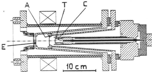
Fig. 3. Metal vapour ion source MEVVA.<sup>2</sup> C, solid cathode made from the material yielding the desired ion species. T, triggering electrode. A, ring anode. E, triode extraction system.
