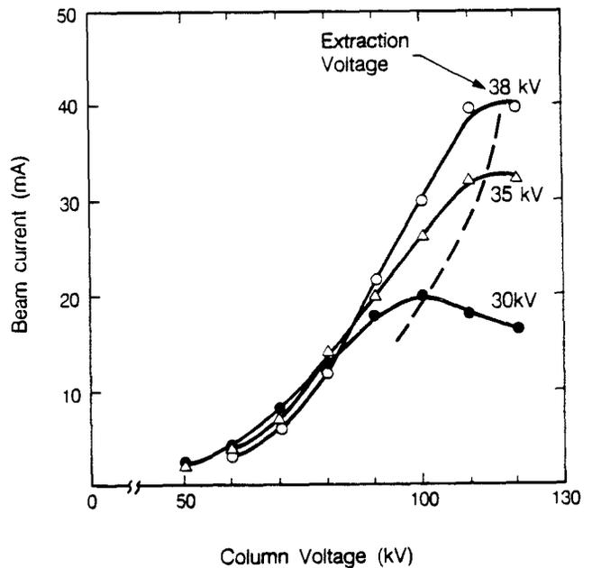
Fig. 6. Beam current measured at the ground side of a high-voltage gap versus gap voltage, with extraction voltage as parameter. The broken line indicates matched conditions that yield maximum transported current for every extraction voltage. The beam consists of 58 % U 4+, 29 % U 3+, and minor shares of other uranium charge states. From Ref. 9.
