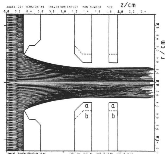
Fig. 4. High-brightness extraction system, designed with the aid of the simulation code AXCEL-GSI.<sup>11</sup> The two cases show electrode shapes optimized for either highest beam current within 20 mrad divergence half-angle (a) or for lowest divergence (b). The extraction voltages of +50 kV and -4 kV (screening voltage) are well tolerated by the 6-mm gap<sup>1</sup>.
