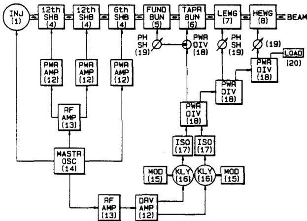
Figure 1. Linear accelerator block diagram.
