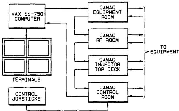
Figure 4. Control system block diagram.
