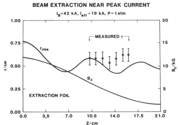
Figure 7: The rms radius calculated with DYNADISC. The solid circles with the error bars are the experimental envelope measurements with the radiochromic foils.
