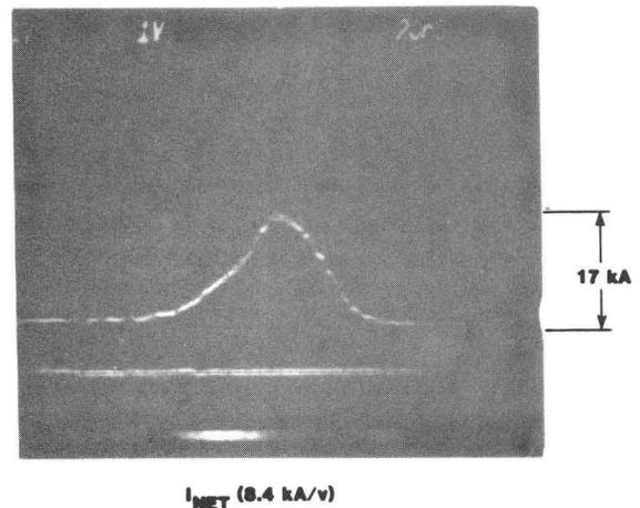
Figure 6: Net current waveform for a 40-kA beam current extracted beam.
