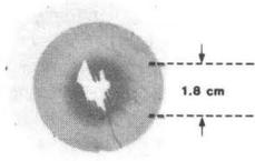
Figure 3: Beam envelope on radiochromic foil inside the accelerator. The part of the foil enclosed by the beam annulus is carbonized.
