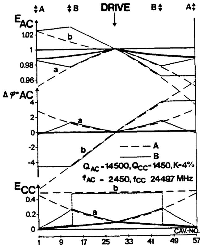
Fig. 3.: Field levels in the AC's and CC's and phases (mod.  $\pi$ ) of the AC's in a standard section. Solid line: structure well tuned, dashed lines: plunger-cavities detuned (A-end tuners, B-middle tuners). Detuning was  $++6.5\text{MHz}$  (a) and  $-6.5\text{MHz}$  (b).
