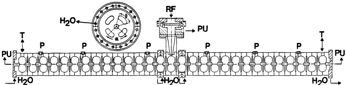
Fig. 1.: The standard MAMI-section (P-probe, PU-pump, T-Tuner)
