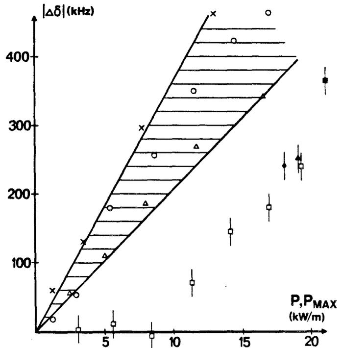
Fig. 4.: Range of slopes of reversible change of the passband gap  $\delta$  with power ( $P, -|\Delta\delta|$ ) and permanent changes measured at zero power after cycling to  $P_{MAX}$  ( $+|\Delta\delta|$ ).
