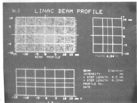
Fig. 7. A low-intensity beam profile with noises; after integration along x- (y-) axis, the y- (x-) intensity distribution becomes clear.
