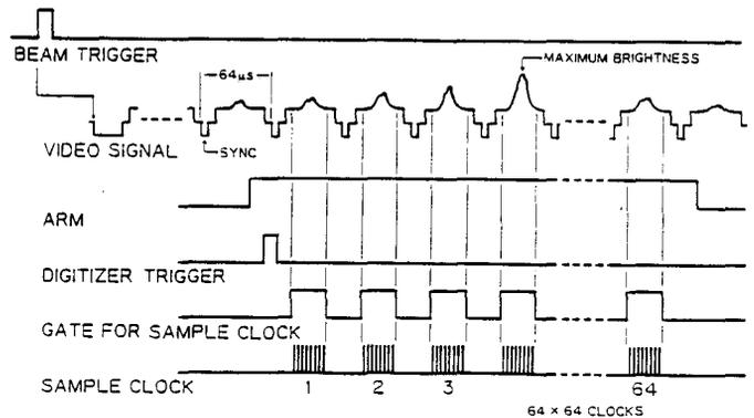
Fig. 2. Gate timing for digitizing the video signal from a TV camera viewing the beam on the screen. Only a narrow area of the screen image effective to observe the beam is digitized and stored in the buffer memory of the transient digitizer.
