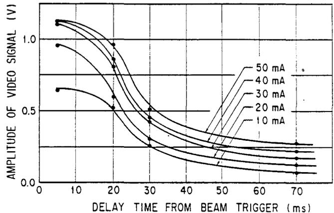
Fig. 3. Peak amplitude of the video signal as a function of the delay time from the beam trigger. Measurement was carried out at the peak current of the beam: 10, 20, 30, 40 and 50 mA. Beam pulse width: 0.8 us. Beam repetition rate: 1 pulse per second.
