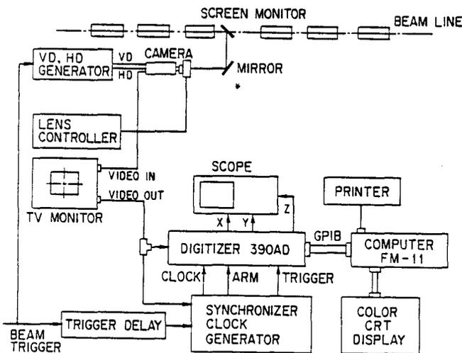
Fig. 1. Hardware configuration of the image processing system for the beam profile monitor.
