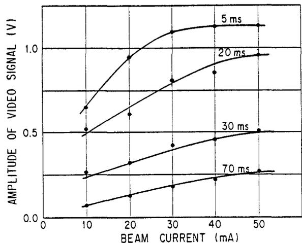
Fig. 4. Peak amplitude of the video signal as a function of the peak current of the beam at delay times from the beam trigger 5, 20, 30 and 70 ms. The data points are the same as those in Fig. 3.
