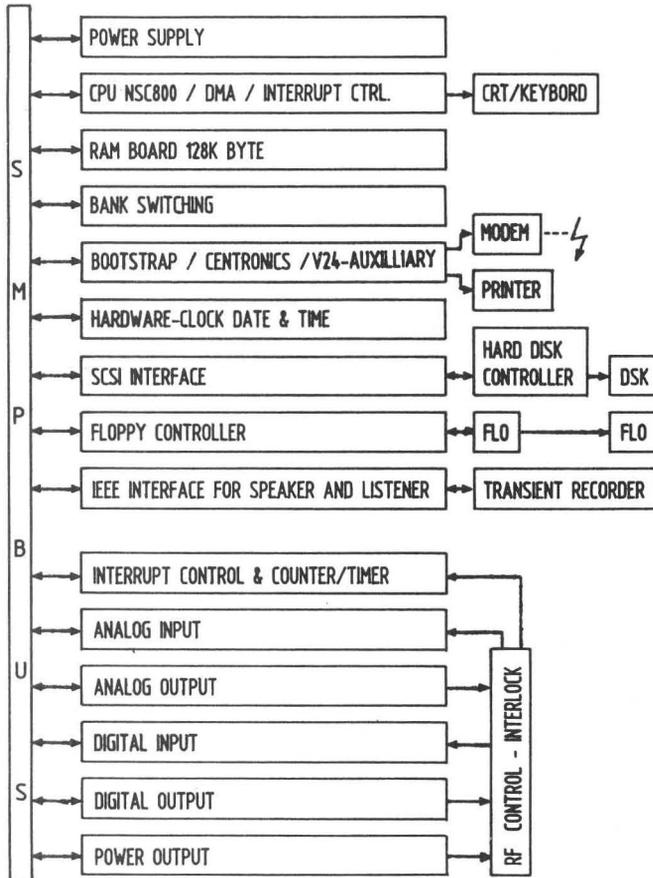
Fig. 3 Internal Structure of the SMP-System
