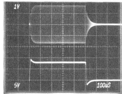
Fig. 4 RF output pulse and its control signal
