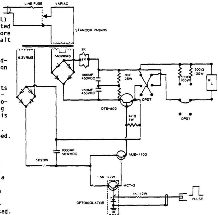
Fig. 2. Electronics for taut-wire pulser.
