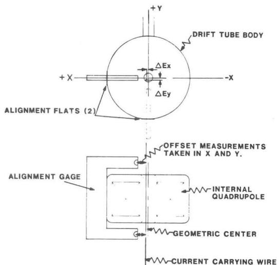
Fig. 4. Alignment jig for measuring magnetic-axis offset.
