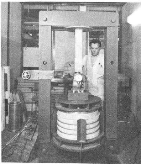
Fig. 8b. Same as Fig. 8a, but with load of 15 tons applied.
