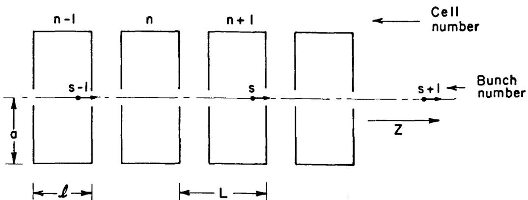
Fig. 2. Uncoupled chain of cylinders with small holes as a linac model.
