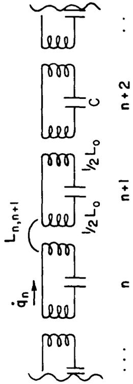
Fig. 4. Equivalent circuit for deflecting modes in a linac model with cell-to-cell coupling.
