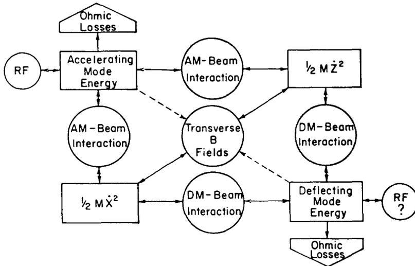
Fig. 1. Energy flow among the various degrees of freedom in the linac-beam system is shown by the solid lines.
