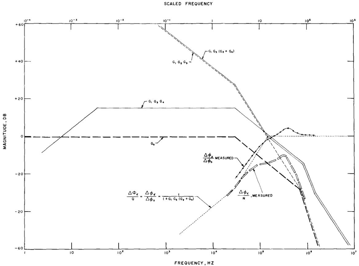
Fig. 8. Transfer functions for the rf phase control loop in Fig. 7.
