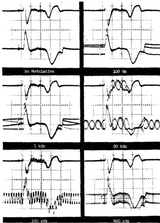
Fig. 5. Behavior of system in Fig. 3 when modulated by "noise" signal, corresponding to  $10^\circ$  peak-to-peak, added to varactor bias voltage,  $\Delta V_B$ . (Top traces: phase error  $\Delta\phi_E$ ,  $8^\circ/\text{cm}$ ,  $50 \mu\text{sec}/\text{cm}$ ; bottom traces:  $\Delta V_B$ ,  $0.2 \text{ V}/\text{cm}$ ,  $50 \mu\text{sec}/\text{cm}$ .)
