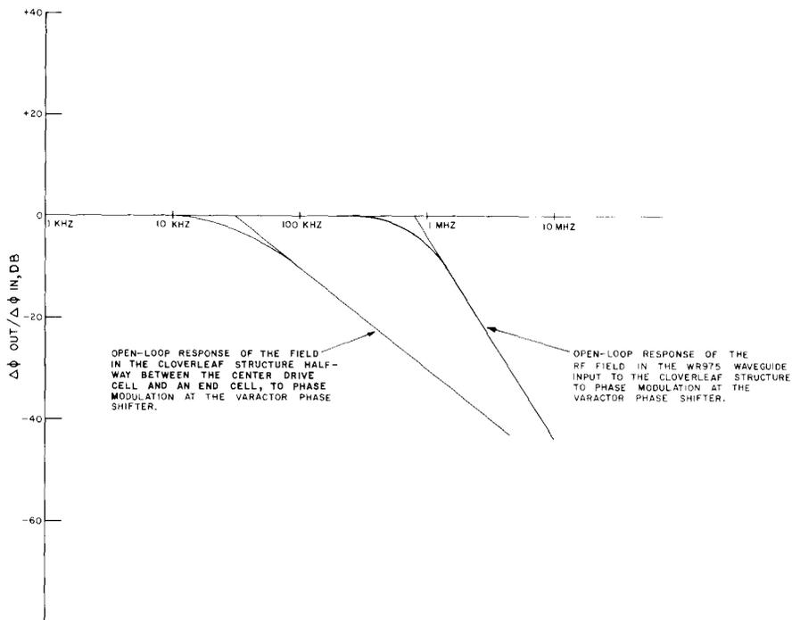
Fig. 2. 805-MHz rf power chain open-loop phase modulation characteristics.
