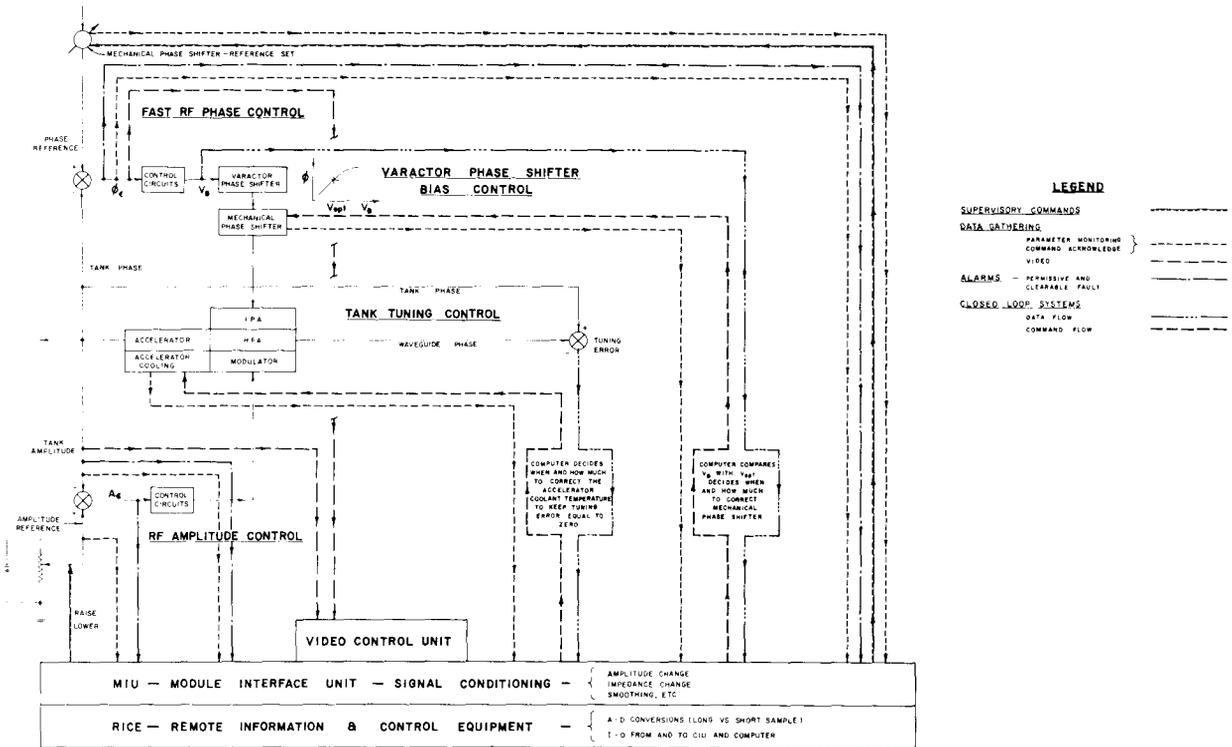
Fig. 9. Interplay between the fast rf phase and amplitude control systems and the central control system, which is based on a real-time control computer.
