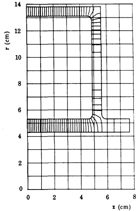
Fig. 10. Computed electric field lines for coaxitron model with extended anode.
