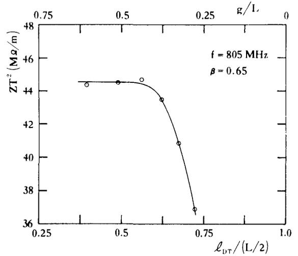
Fig.5. Variation of Shunt Impedance  $ZT^2$  with drift tube length for cavities of Table I.
