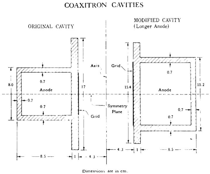
Fig. 9. Computational models of coaxitron cavities.
