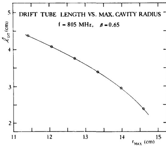
Fig.4. Relationship between  $l_{DT}$  and  $r_{MAX}$  for cavities of Table I.
