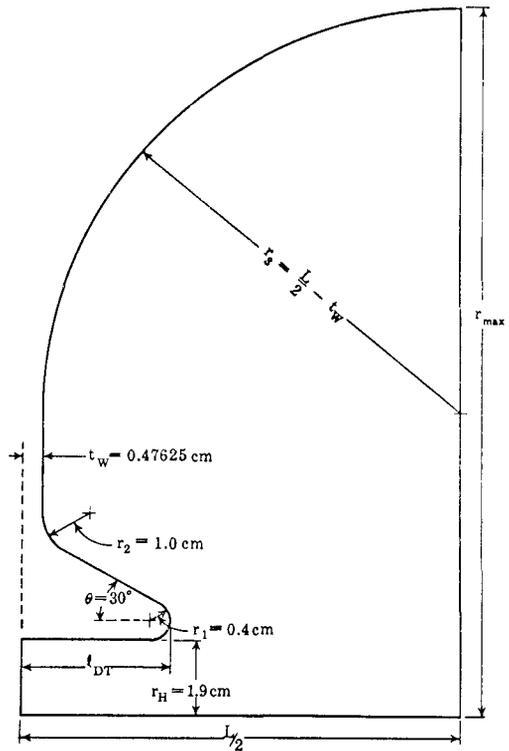
Fig.2. Shaped 805 MHz Proton Linac Cavity
