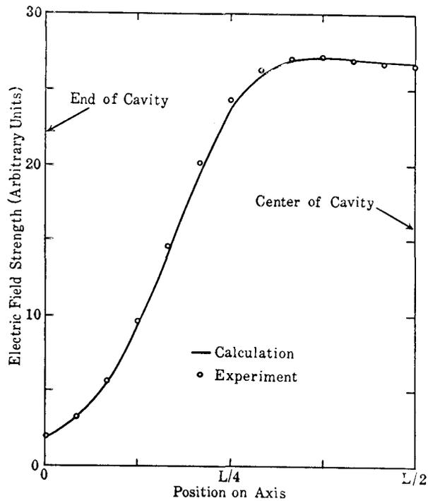
Fig.3. Electric field on axis of cavity of Table II.
