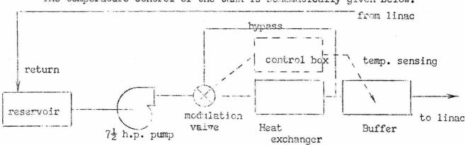
The temperature control of the tank is schematically given below.
