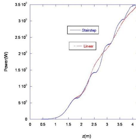
Fig. 5. FEL peak power versus distance for both the stair-step (blue) and linearly (red) tapered wigglers.
