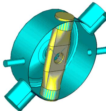
Fig. 3. The LANL single-spoke cavity at 350 MHz. The fundamental and HOM couplers are mounted on the side.
