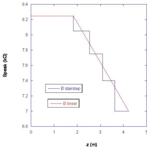
Fig. 4. Magnetic field profiles of both stair-step (blue) and linearly (red) tapered wigglers.
