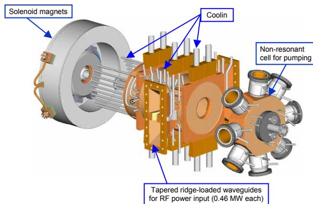
Fig. 2. LANL/AES NCRF high-average-current gun.
