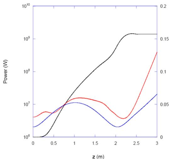
Figure 1: Plot of peak power on log scale (black), FEL beam radius (red) and electron beam radius (blue) versus wiggler length in a scalloped electron beam FEL.
