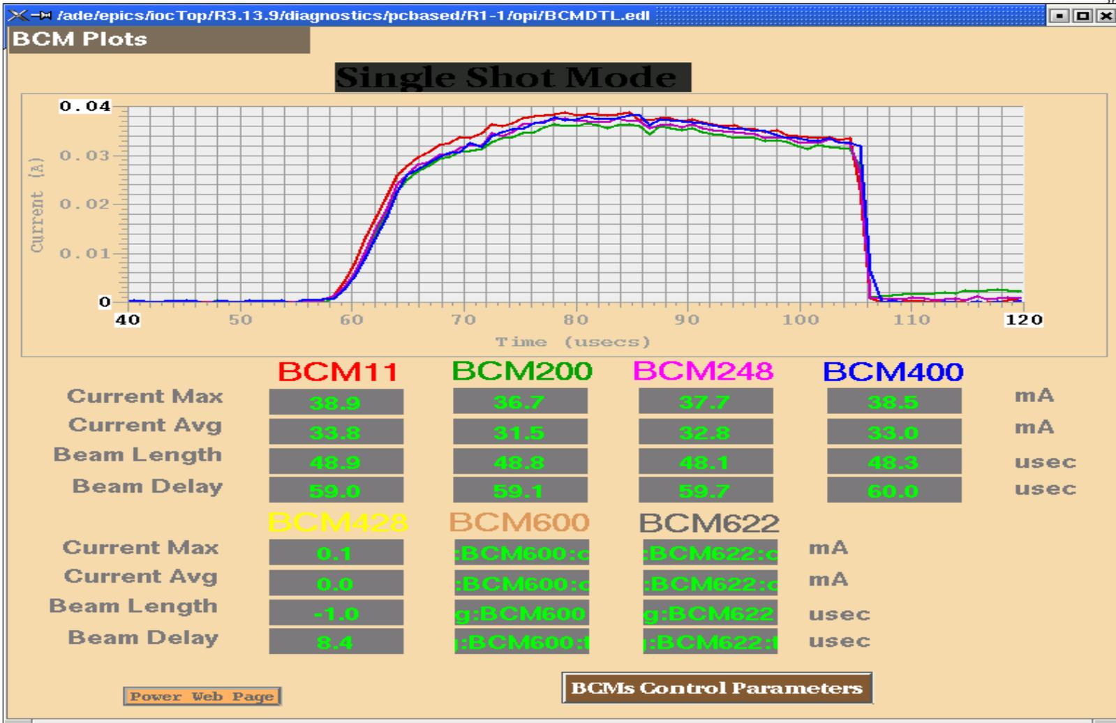
Beam current after MEBT (red), DTL tank1 (green), DTL tank2 (pink), DTL tank3 (blue)
