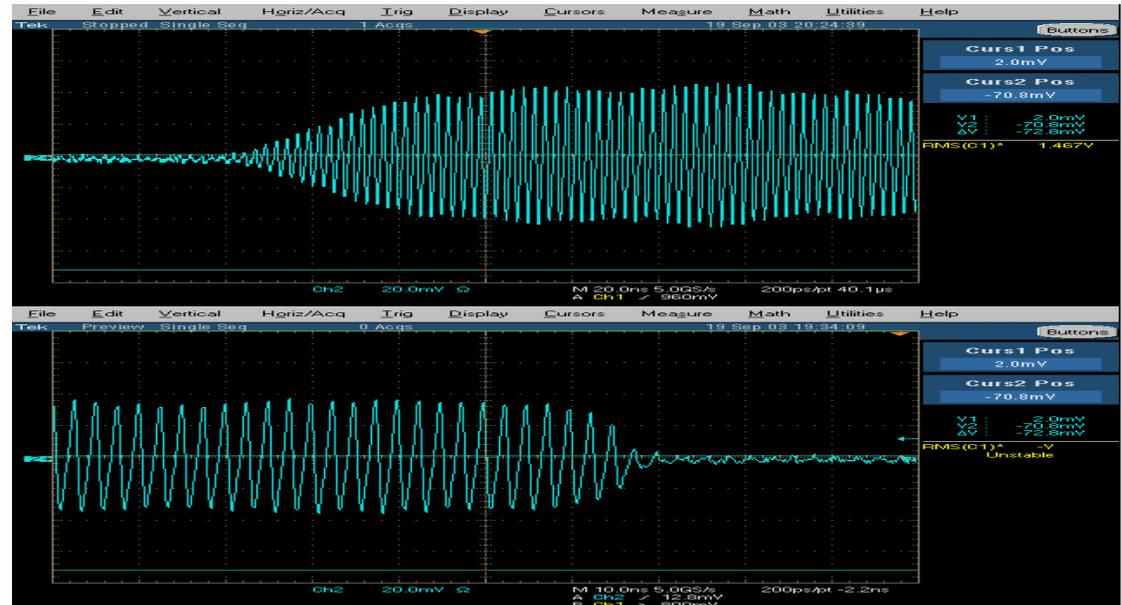
Measured effect of chopper on the beam (LEBT top, MEBT bottom)
