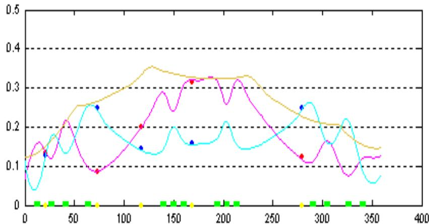
RMS beam envelope in MEBT. Simulation (solid) and wire scanner measurements (dots).
