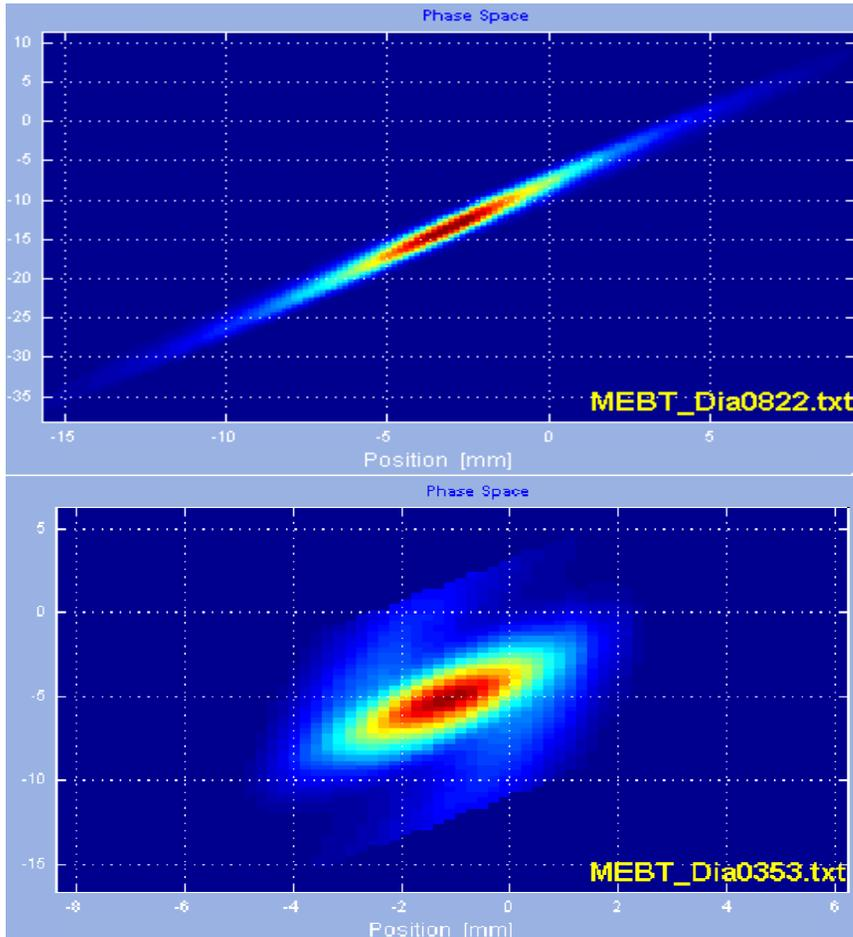
**Beam emittance after MEBT. Vertical (top) and horizontal (bottom)**
