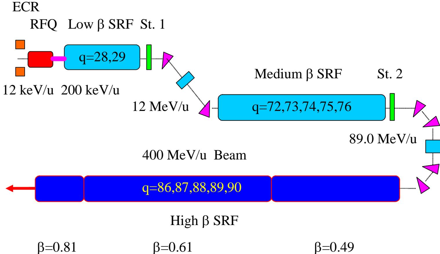
**Baseline Design: 393 SC cavities of 9 different types arrayed in three linac sections**
