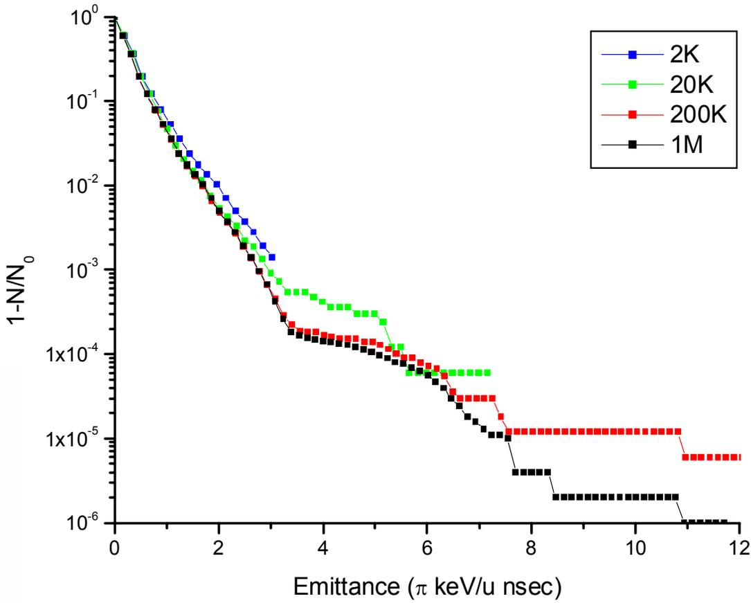
***Fraction of particles outside of a given longitudinal emittance as a function of the emittance.***
