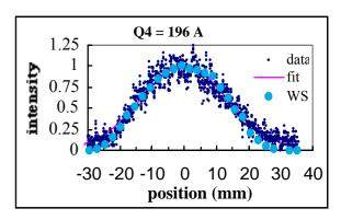
The profile measurement data agree within < 10%, while the BIF profiles show always a slight broadening, maybe caused by a space charge effect
