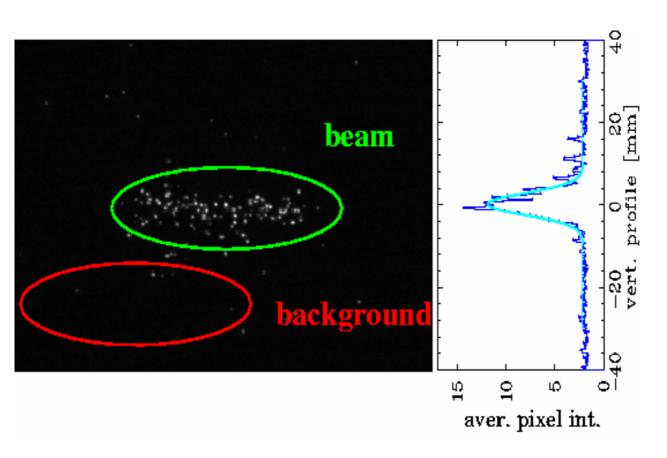
Image of a 200 μs U<sup>28+</sup> beam with I=700 μA recorded during one UNILAC macro-pulse with a vacuum pressure of about 10<sup>-5</sup> mbar. The two dimensional image from the intensifier (left) and the projection for the vertical beam profile (right) is shown
