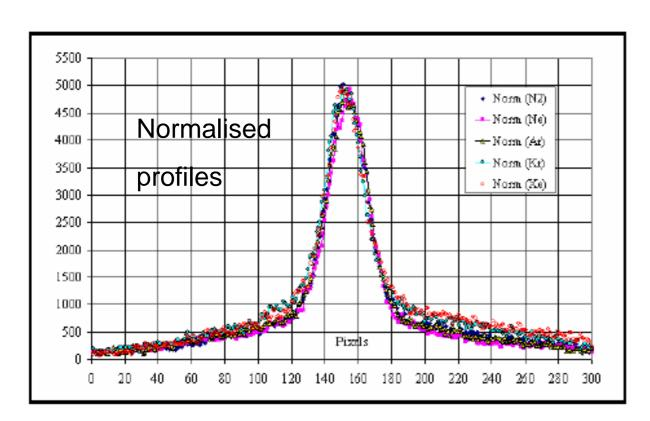
Measured profiles have the same geometrical shape for all gases at the same pressure,
