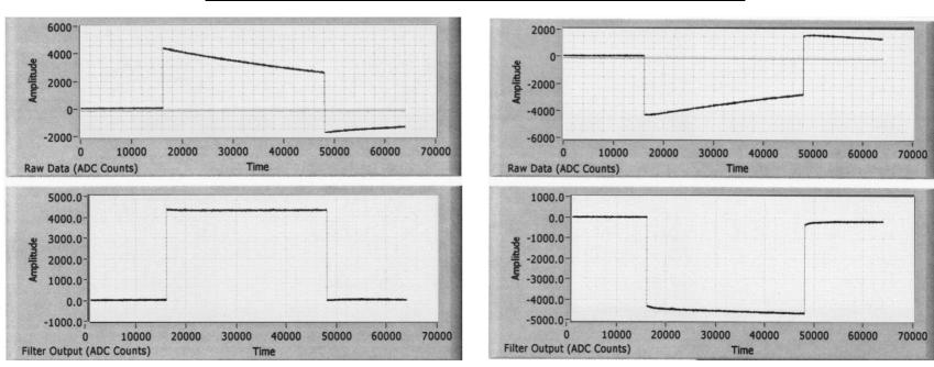
Measurements verify the function of the filter (left pictures) but pulses in the opposite direction (right pictures) indicate a slight variation of the transformer's inductance due to hysteresis effects  $\rightarrow$  *Solution:* online calibration using a test pulse in the gap between two beam pulses, implementation of evaluation and correction in a FPGA/DSP
