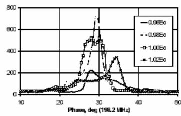
Bunch shapes at the exit of the first tank of INR linac for different accelerating fields
