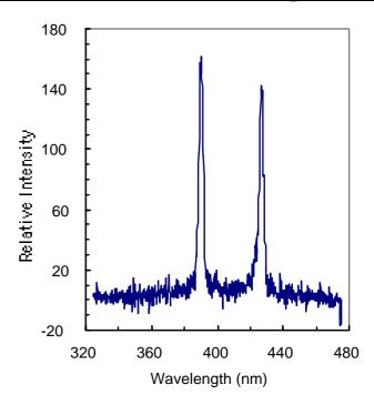
Spectrum measured by D. Gilpatrick (LANL),  $N_2$  partial pressure: 5 x10<sup>-6</sup> Torr, excited by a MeV proton beam  $\Lambda_{-}\Lambda_{-}$
