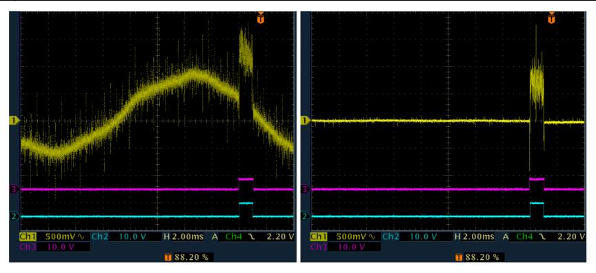
Analog signal processing is the first step to get rid of EM interferences, here: clamping technique
