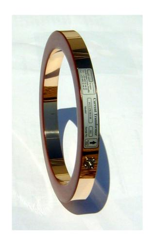
Current transformers must have <1 ns rise time and droops of 0.1%/ms due to varying beam parameters along the accelerator facility  $\rightarrow$  not achievable with a normal (active-)passive transformer ( $\tau_r$  0 rLC,  $\tau_d$  0 L/R)
