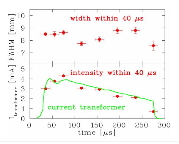
A measurement of the width variation during macro pulse (each data point taken in **one** pulse) is shown.
