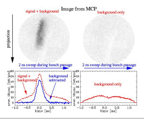
Typical image (inverted colour) from the MCP for a 60 µA Au<sup>25+</sup> beam averaged over 16 macro-pulses with 1 ms length. The background only is displayed on the right side.
