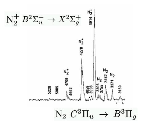
Spectrum measured by R.H.Hughes, 1961, using 200 keV protons
