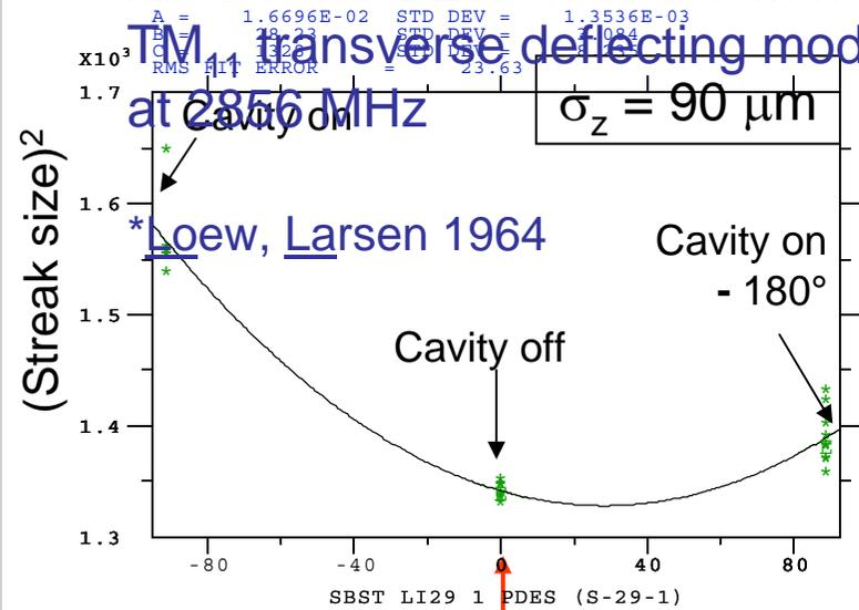
Asymmetric parabola indicates incoming tilt to beam
