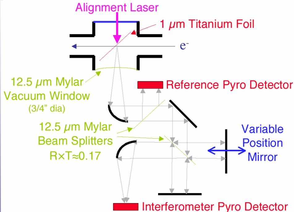
Transition radiation is coherent at wavelengths longer than the bunch length,
