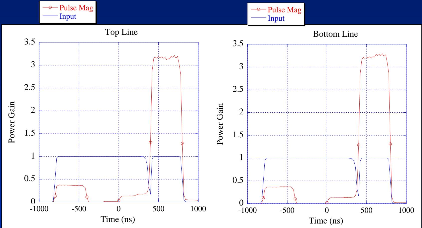
Theoretical gain for a compression ratio of four is 3.44 (lossless).
