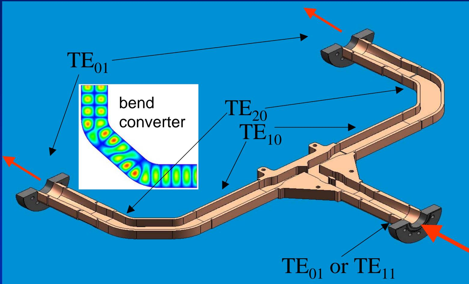
For either incident mode, power is evenly divided between the two output ports, which launch  $TE_{01}$ .
