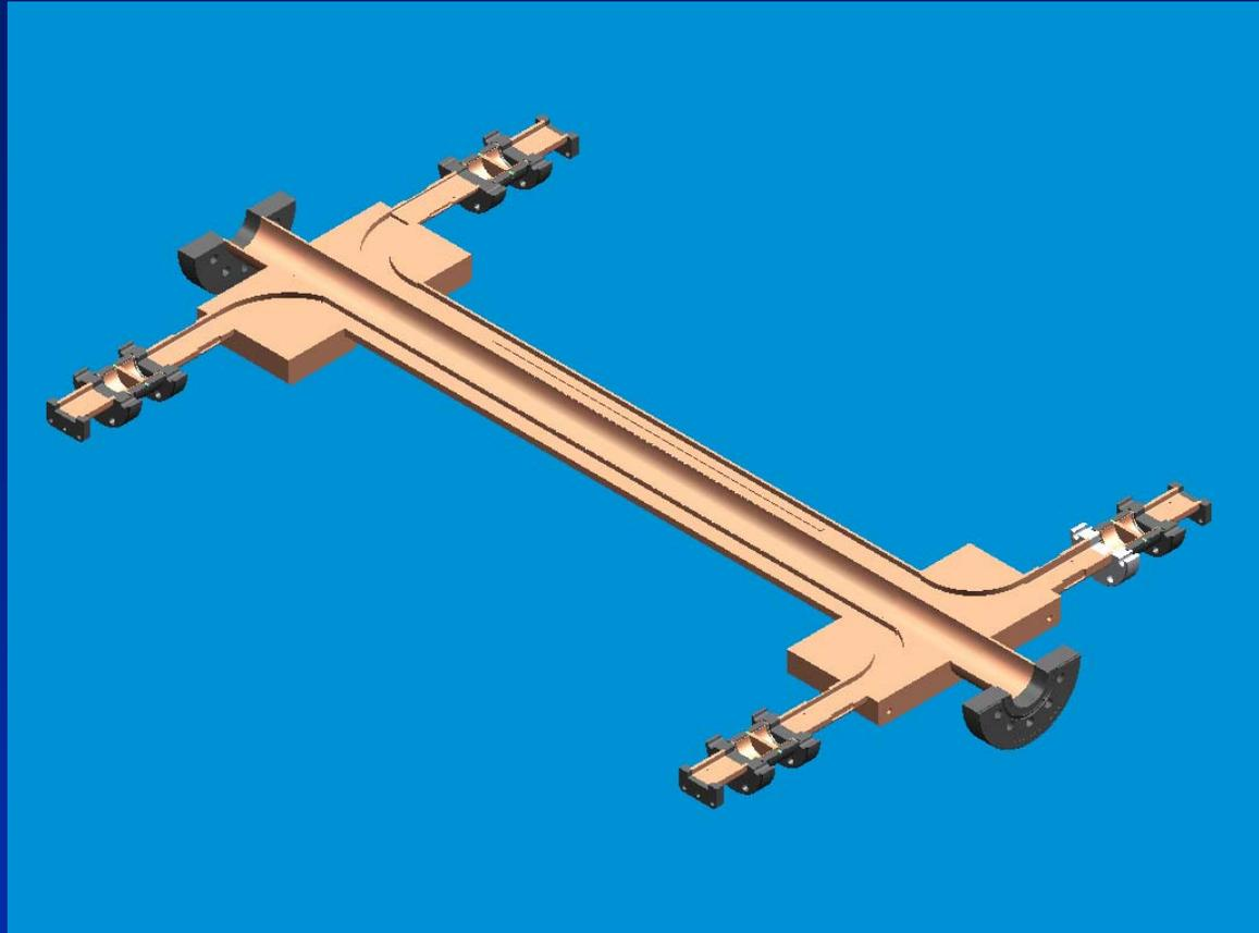
• waveguide sizes chosen to match wavelengths in side waveguides to circular waveguide modes.
