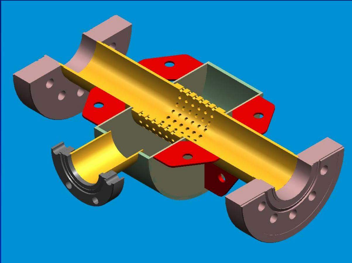
The hole pattern is designed to cancel any coupling or reflection for the  $TE_{01}$  and  $TE_{11}$  modes.
