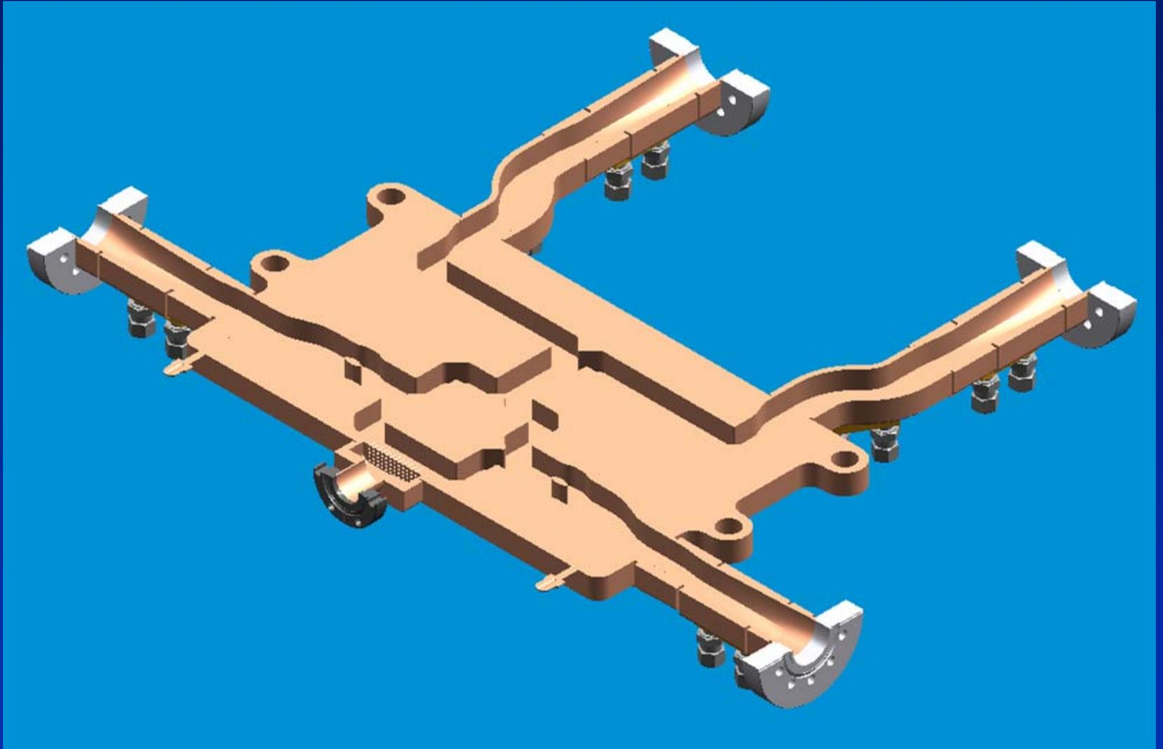
equivalent to three planar hybrids on one single substrate
