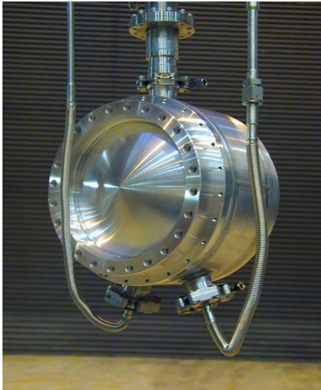
Prototype LH<sub>2</sub> absorber
