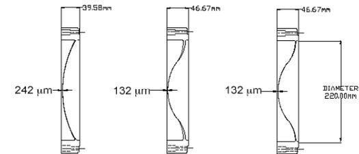
— use photogrammetry to characterize window behavior and verify FEA calculations (LH<sub>2</sub> safety requirement)
