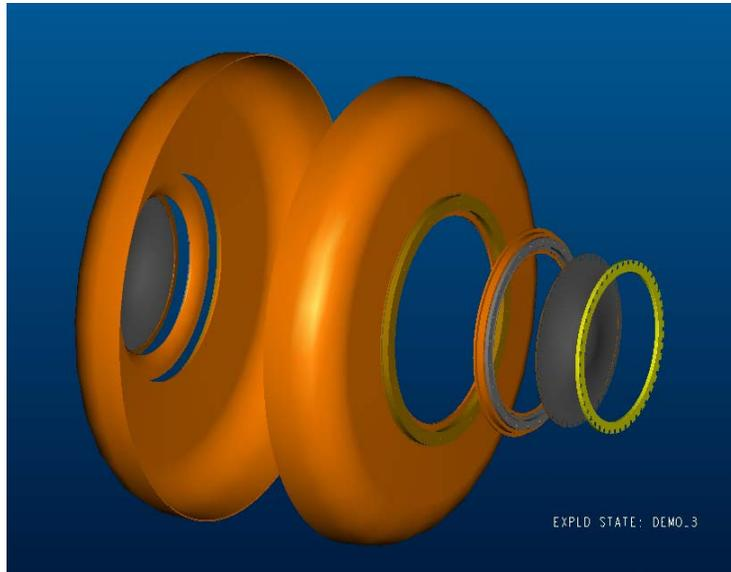
Exploded view of 201 MHz cavity
