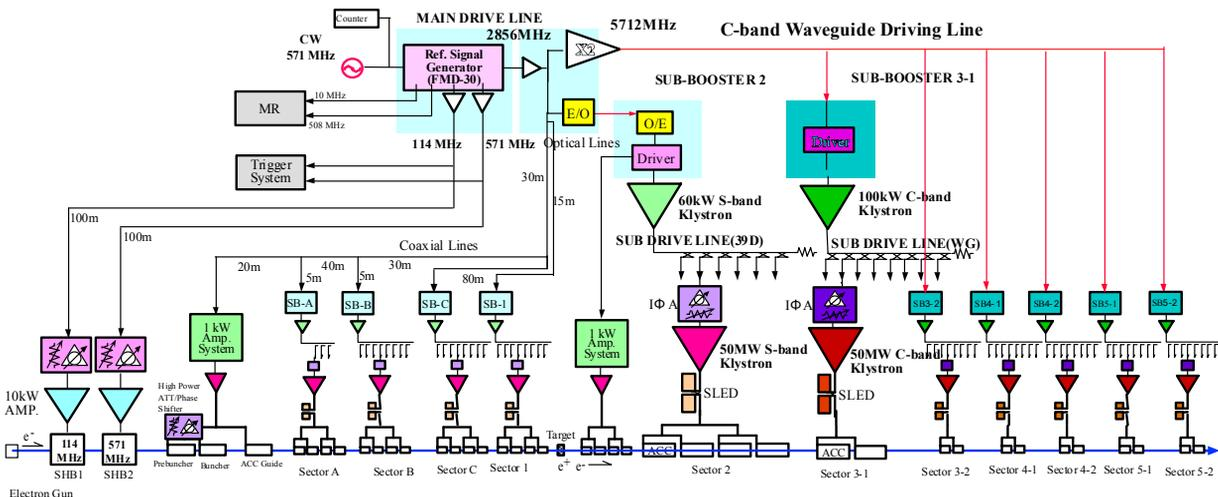
Figure 9: Rf system planned for the linac upgrade.
