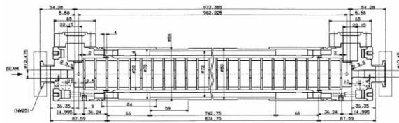
Figure 12: C-band acceleration structure.
