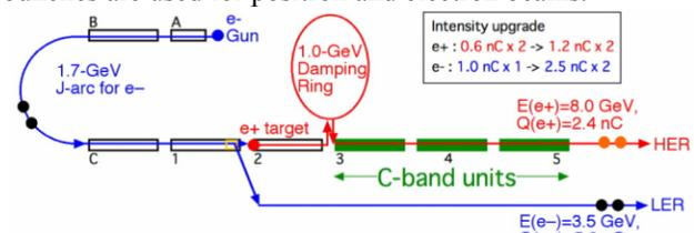
Figure 7: Layout of the linac upgrade for SuperKEKB.
