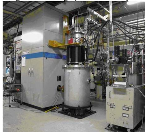
Figure 15: Photograph of the C-band unit installed in the klystron gallery.
