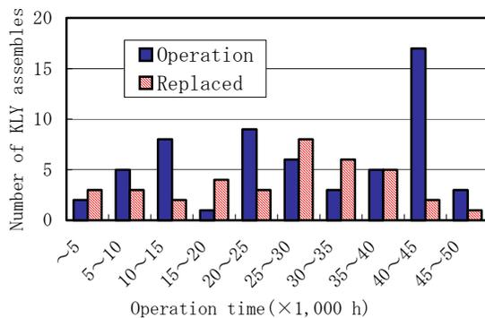
Figure 4: Operation and replaced time of the klystron assemblies. The assemblies installed at the beginning of the KEKB were used for more than 40,000 hours.
