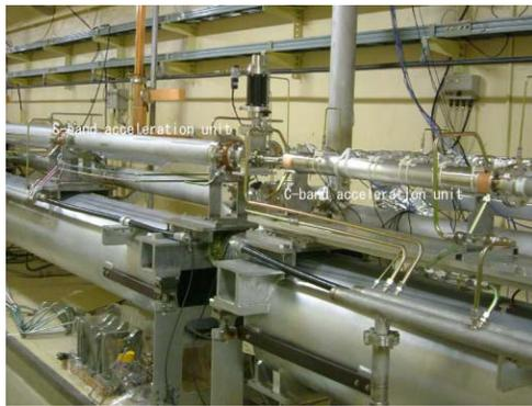
Figure 16: Photograph of the C-band acceleration unit installed in the beam-line.
