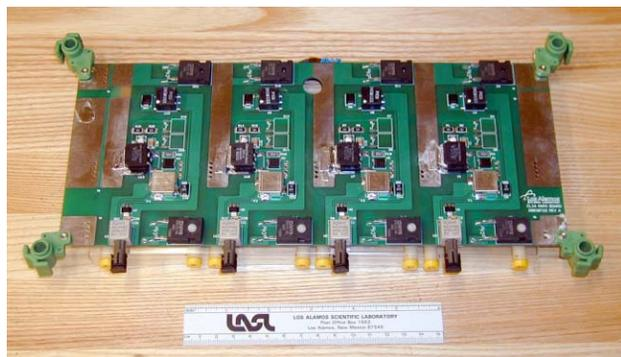
Figure 4: Photograph of a single Marx circuit board showing 4 IGBTs, 4 optical receivers, and 8 charging diodes.
