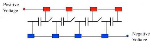
Figure 3: Schematic of a basic Marx-generator module.
