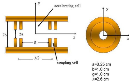
Figure 1: Cross sections of a 17-GHz linac structure.
