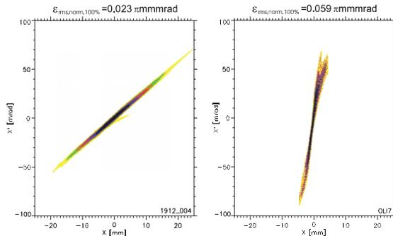
Figure 3: Measured beam emittance behind the differential pumping stage (left) and behind the LEBT – system (right) at I=8.4mA.
