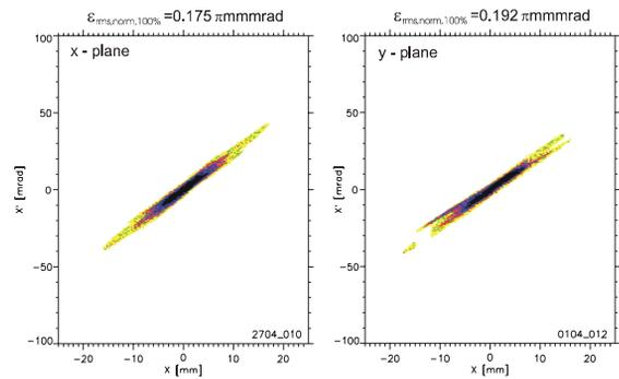
Figure 4: Measured beam emittance behind the RFQ in x-plane (left) and in y-plane (right), beam current I= 1,15 mA.
