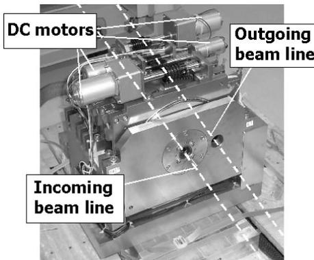
Figure 3: Fabricated 2<sup>nd</sup> prototype PMQ.
