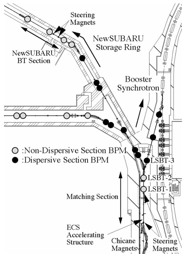
Figure 2: Location of installed dispersive section BPMs.
