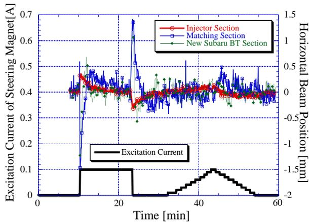
Figure 4: Example of horizontal position feedback control.
