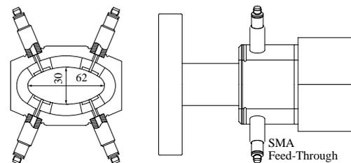
Figure 1: Schematic drawing of dispersive section BPM.
