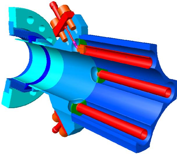
Figure 2: Sectional view of a TTF2 stripline-BPM.
