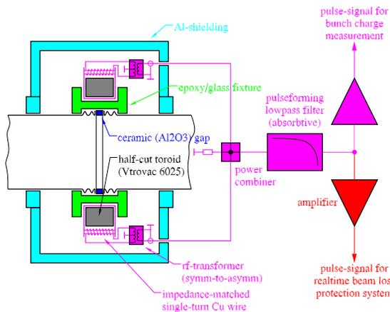
Figure 4: Toroidal transformer with front-end electronics for beam intensity measurements.
