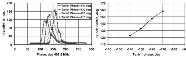
Figure 7: Bunch phase position for different Tank 1 phases.
