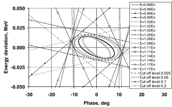
Figure 9: Phase ellipses at the entrance of Tank 1 for different cut off levels (The tangents are shown for 0.025 cut off level).
