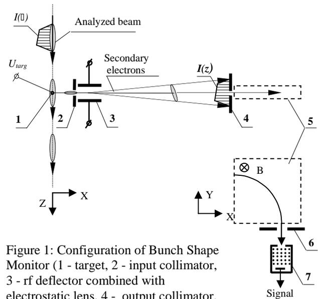
Figure 1: Configuration of Bunch Shape Monitor (1 - target, 2 - input collimator, 3 - rf deflector combined with electrostatic lens, 4 - output collimator, 5 - bending magnet, 6 - collimator, 7 - Secondary Electron Multiplier).
