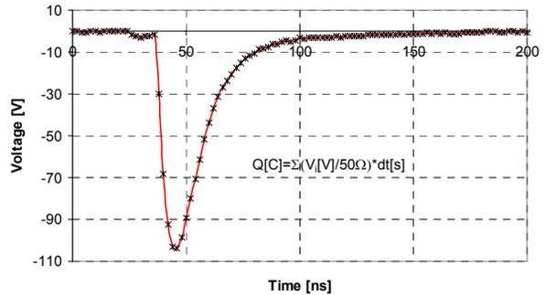
Figure 5: Signal recording for charge measurements: calibration is  $1 \text{ nC} / 2 \cdot 10^7 \text{ V.s}$ .
