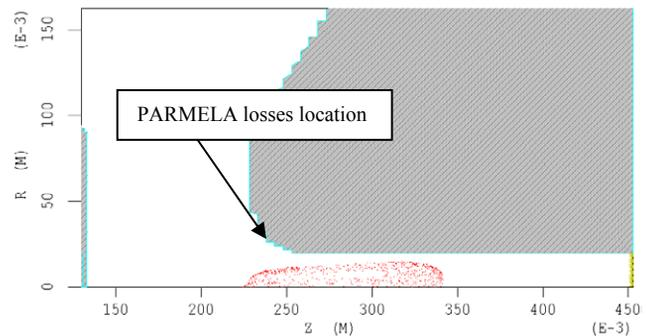
Figure 8: Extracted charge propagation from PARMELA simulations.
