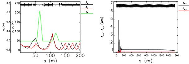
Figure 3: Twiss parameters around BCs (left) and projected emittances along XFEL linac (right).
