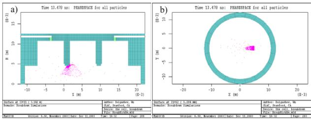
Figure 1: Snapshots of MAGIC3D screen with geometry of the travelling wave structure: electrons (red), and copper ions (magenta). a)  $(r, z)$  plane, b)  $(x, y)$  plane. Beam and rf energy move left to right in a); emission spot is at right in b), with  $y = 0$ . Emission spot is on downstream half of first iris.
