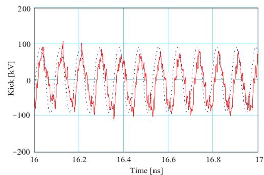
Figure 4: Transverse kick (solid) induced by arc current in a structure cell, after 16 ns. The dashed curve is one tenth of acceleration.
