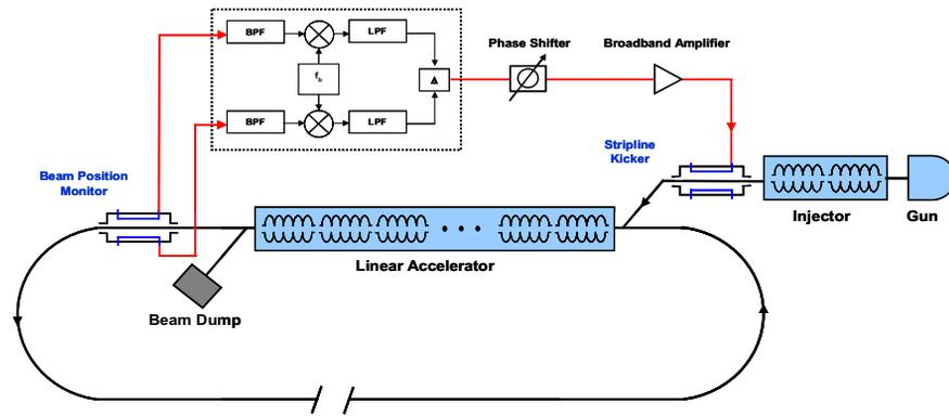
Figure 3: Schematic for an injector beam-based feedback system. A heterodyne receiver mixes down a BPM signal which is shifted in phase, amplified and used to drive a kicker in the injection region.
