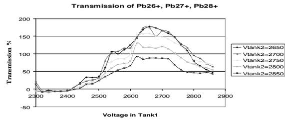
Figure 6: Transmission of three charge states through the LINAC3 IH. For reference the single charge state transmission is 85%.
