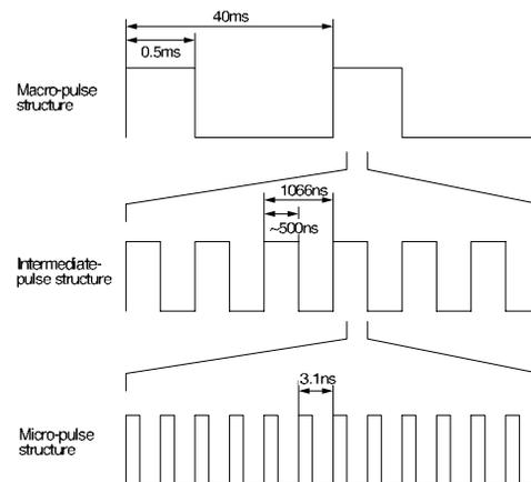
Figure 1: Pulse structure for J-PARC linac (181-MeV injection).
