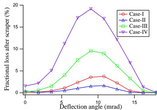
Figure 3: Downstream beam loss vs deflection angle.
