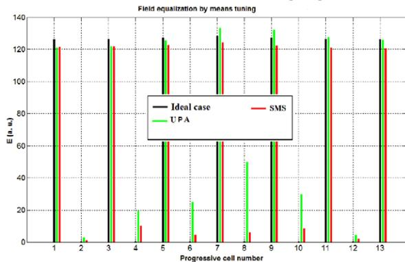
Figure 2. Comparing UPA and SMS,  $f=10\text{MHz}$ .
