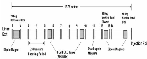
Figure 1: Unfolded layout of the booster transfer line.
