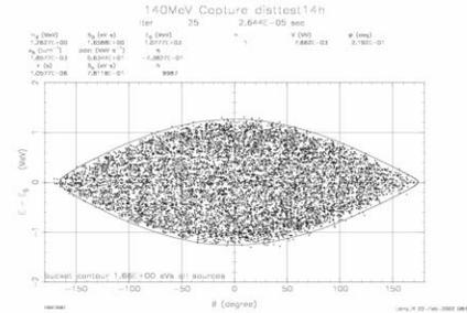
Figure 5: ESME2K simulation results showing the matched beam distribution injected into the booster over 25 turns. The second CCL tank provided ~1.15 MeV of energy variation over a range of 50° of phase as seen by the linac beam.
