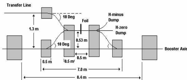
Figure 2: Booster injection region geometry. The final four transfer line quads were adjusted to meet the beam requirements at the foil.
