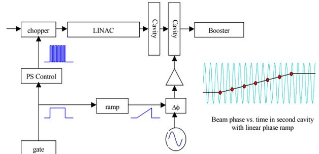
Figure 4: Schematic of the correlated longitudinal painting system. The drive signal to the sweeping cavity is phase modulated with a linearly-increasing phase to sweep the beam across the desired range of phase over the macropulse. The modulation is synchronized with the chopping pattern and the booster RF.
