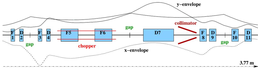
Figure 2: Chopper line and beam envelopes from TRACE3D.
