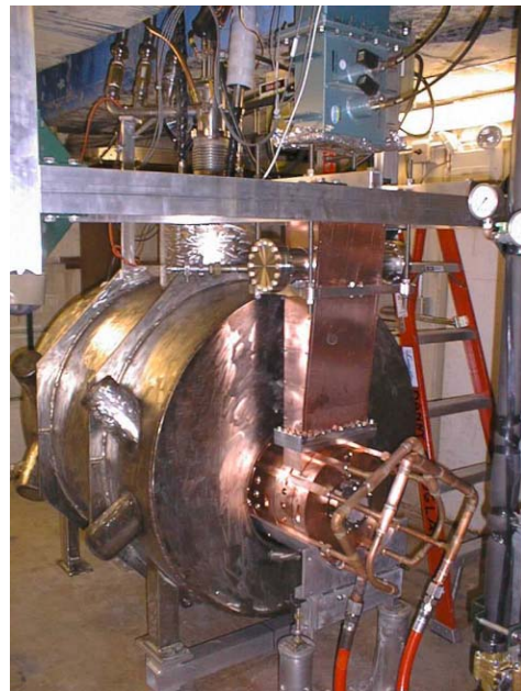
Figure 1: Picture of the open cell test cavity in the Solenoid.
