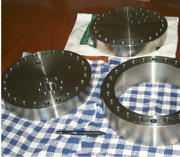
Figure 3: Picture of the Test Cell Stainless Steel Disks and Cylinder before copper plating.
